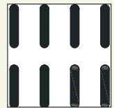
Perforation: .125 in. x .625 in. Open area: 19.5%
